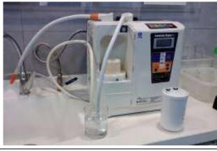
6.Install the filter back and press the clean water again for 3 minutes.
